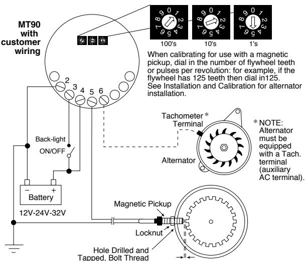
**NOTE:** Gap from face of gear tooth must be enough for gear to move. Rotate gear completely to be sure of minimum, no-touch clearance. See instructions supplied with magnetic sensor.
