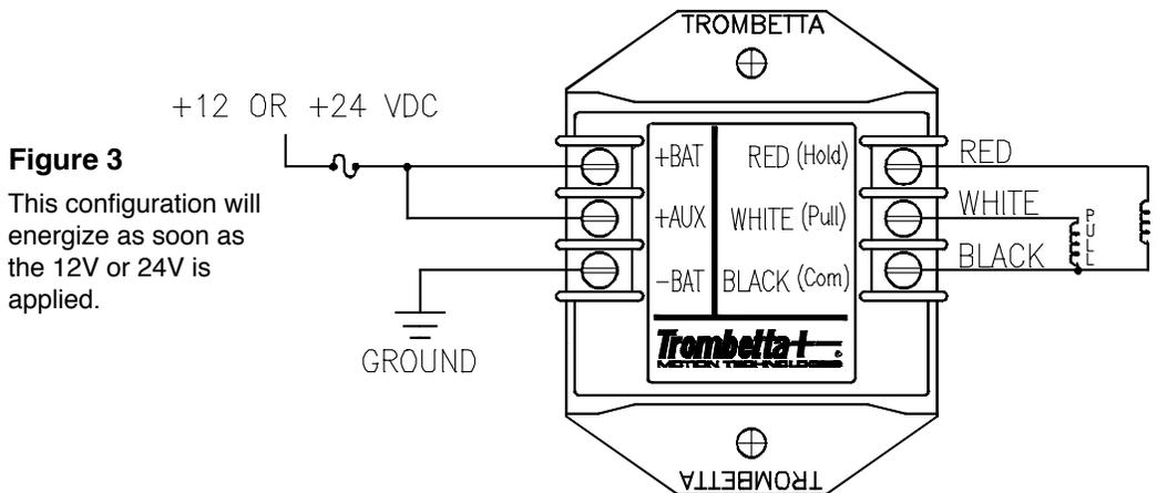
NOTE: When using an S500-A60 module, all of the solenoid connections must connect to the module as shown. Do not connect any of the solenoid leads to another ground point in the system.
