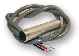
The Model 12 is an air temperature sensor. It is intended for use in applications that monitor slowly changing temperatures. The unit gives approximately  $0.5^{\circ}$  F ( $0.2^{\circ}$  C) resolution when used with an 8-bit analog input.
