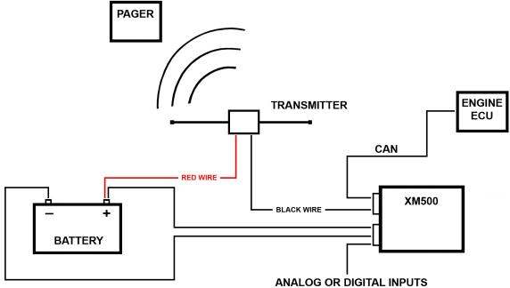
The 2-wire engine pager is available to be triggered by positive or negative contact. The above illustration shows a typical installation utilizing the Murphy XM500 CAN Bus Input/Output Module.
